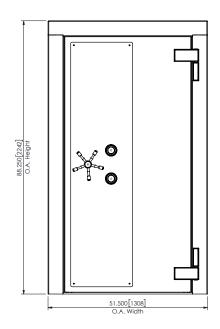
Hamilton's vault doors and frame assembly met the requirements of UL 10C, UL 10B and ULC S104 for a 3-hour fire-resistance rating with hose stream. The Class 1 rating is 30 minute, Class 2 rating 60 minute, & Class 3 rating 120 minute UL security Rating.
